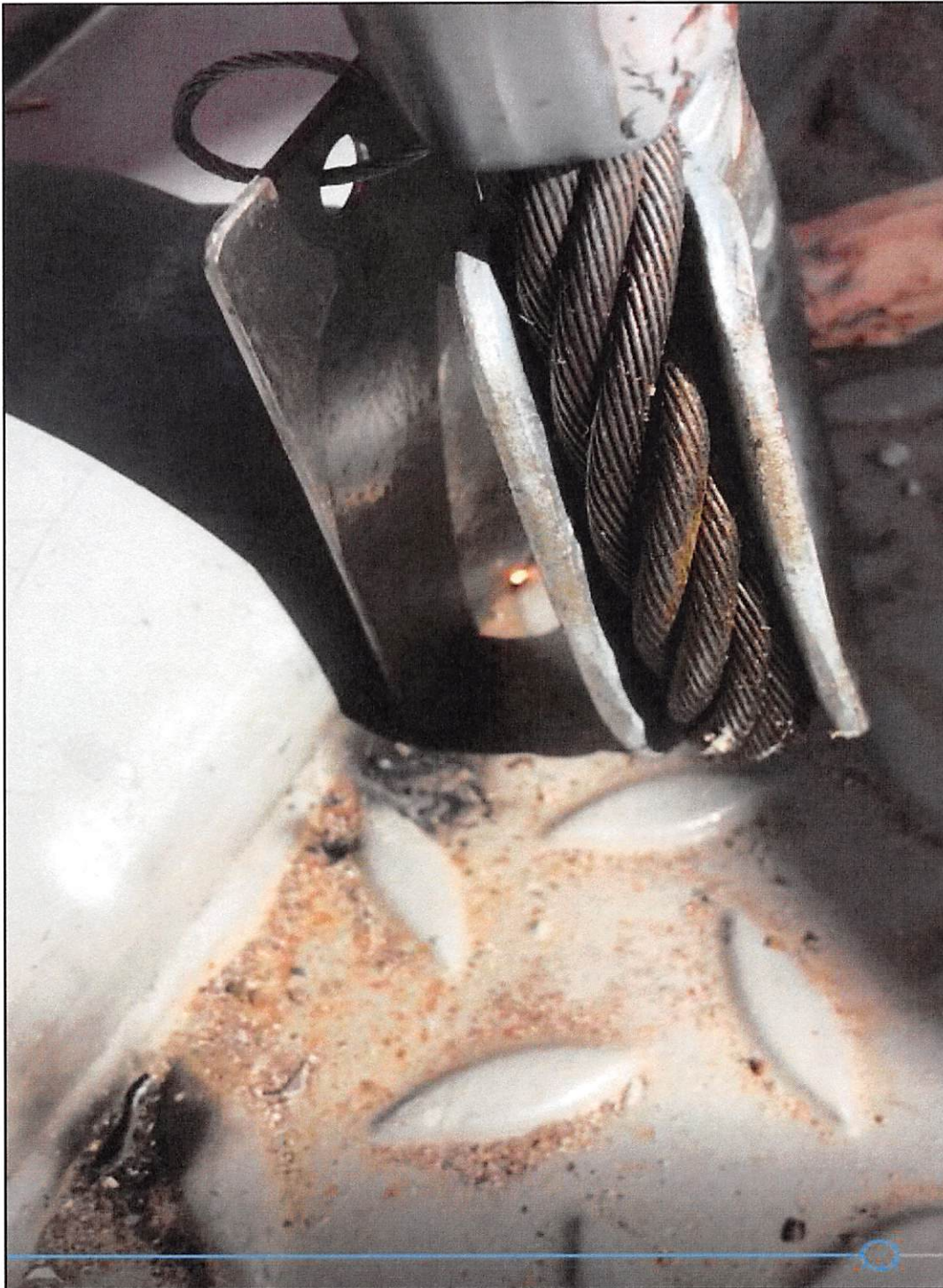
Fig. A1-1b: Arcing cable termination in a hoisting system in a 2.5 V/m field intensity environment. Burn marks can be seen on other places from previous contact.
