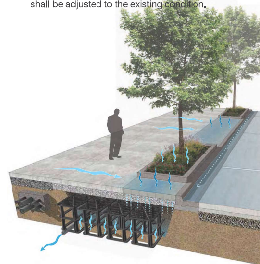
A traditional curb & gutter street with tree pits utilizing soil cells, open planters and stormwater to provide passive irrigation
