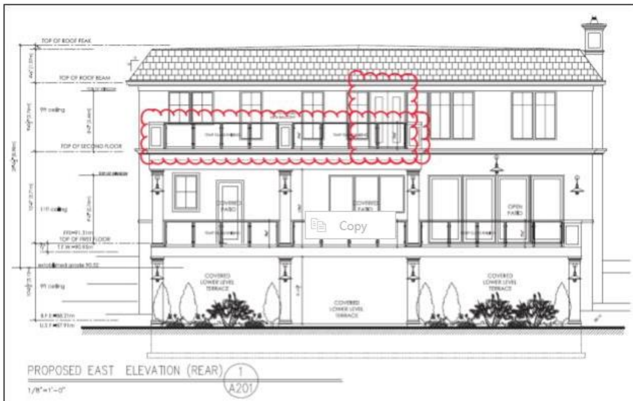
Rear Elevation markups showing balcony elements (i.e. glass railings and doors)
