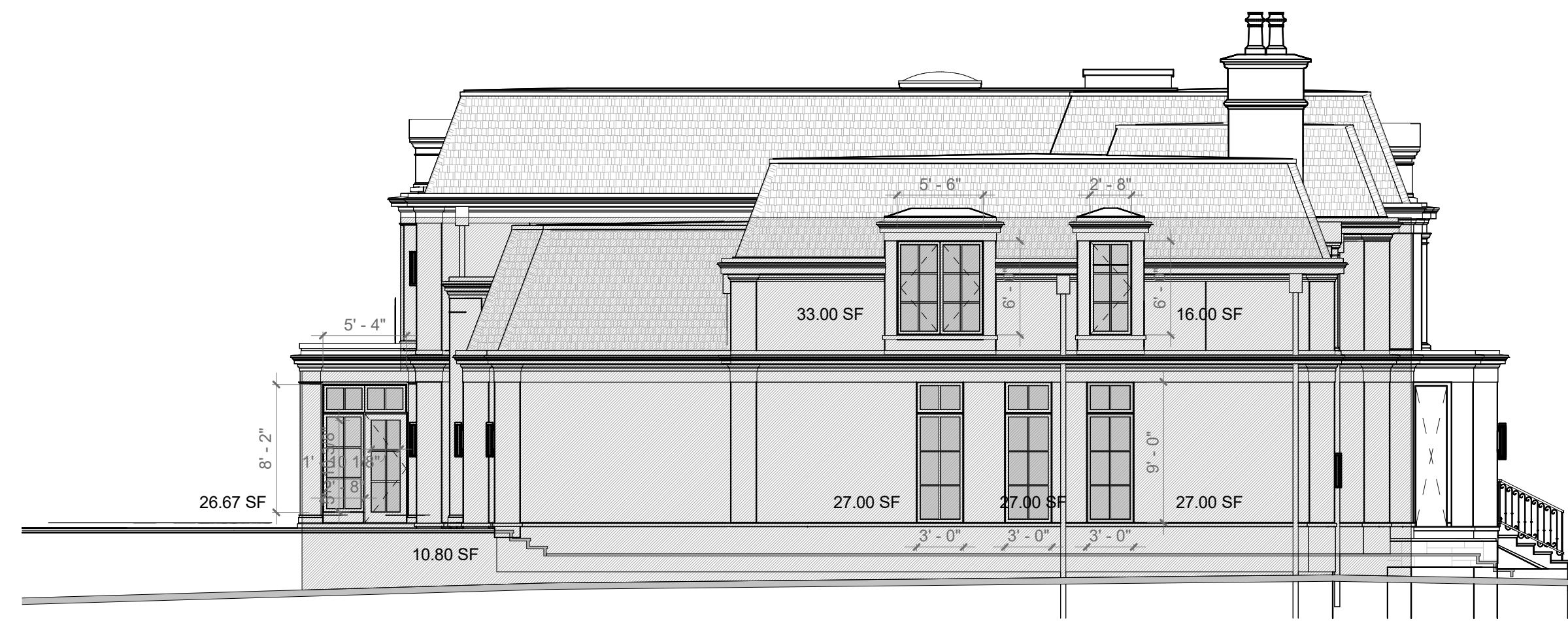
2 NORTH/EAST (SIDE) ELEVATION - UNPROTECTED OPENING CALCULATION A 203 1/8" = 1'-0"
