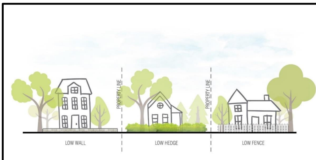
Figure 77: Continuous street edge with porous and low-lying fencing/wall treatments
