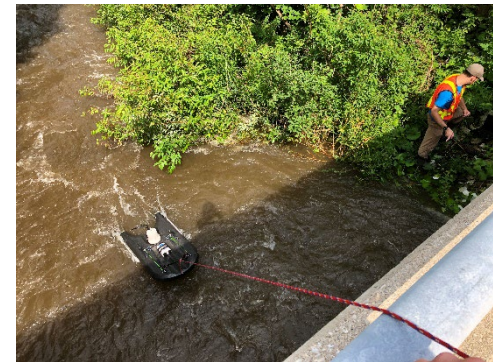
High Flow Measurements – Sixteen Mile Creek at Appleby Line – July 16, 2024
