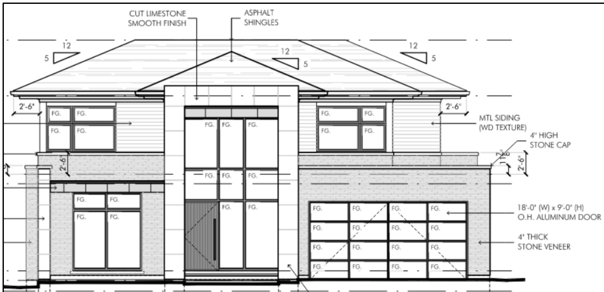
Primary Façade – 1457 Constance Drive
