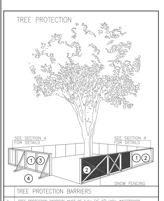
TREE PROTECTION BARRIERS MUST BE 1.2m (4'-0") HIGH. WAFERBOARD HOARDING OR AN EQUIVALENT APPROVED BY URBAN FORESTRY SERVICES. TREE PROTECTION BARRIERS FOR TREES SITUATED ON THE TOWN ROAD ALLOWANCE WHERE VISIBILITY MUST BE MAINTAINED CAN BE 1.2m (4'-0") HEIGHT AND CONSIST OF ORANGE PLASTIC WEB SNOW FENCING ON A WOOD FRAME MADE OF 2"X4"'S.
