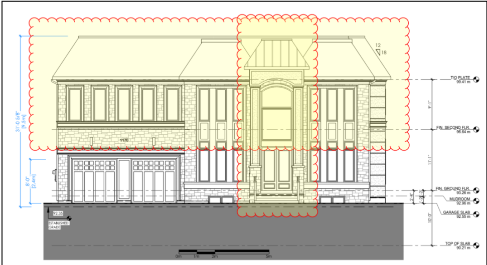
Excerpt of Proposed Front (West) Elevation with emphasized architectural elements – 1178 Wood Place
