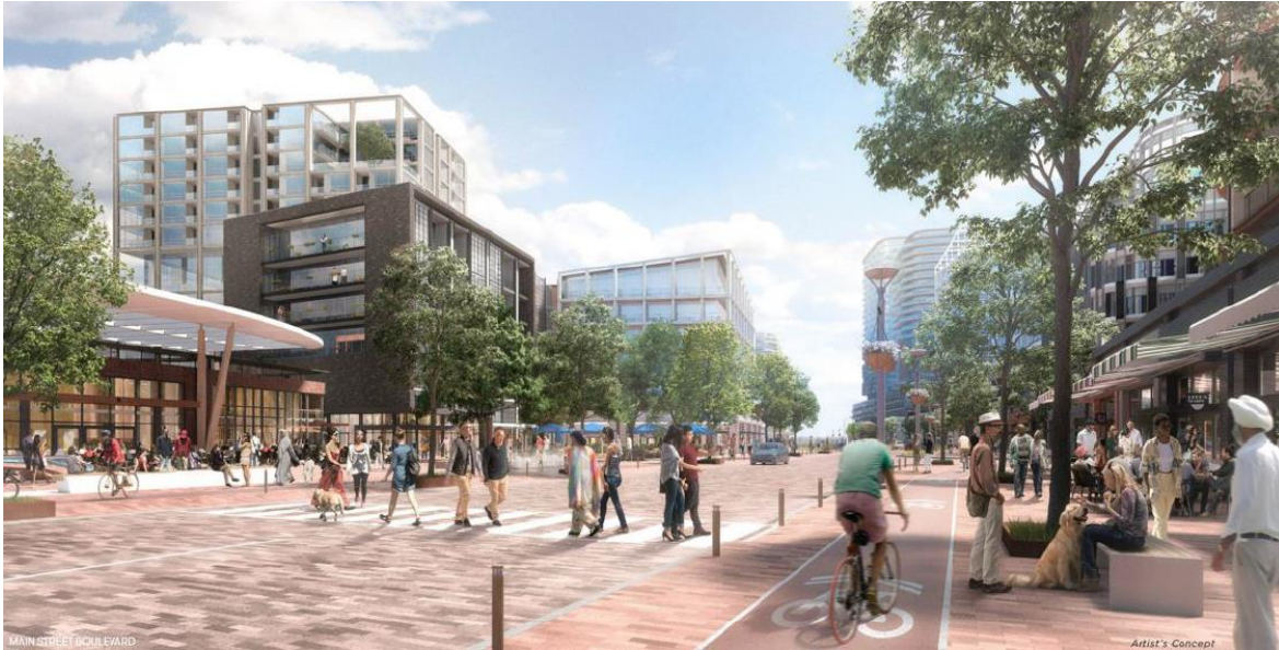
Figure 16: Main Street promenade at Brightwater Mississauga. The two-lane road, bike paths, wide sidewalks, and woonerf design combine to slow traffic and create a comfortable pedestrian-oriented retail corridor
