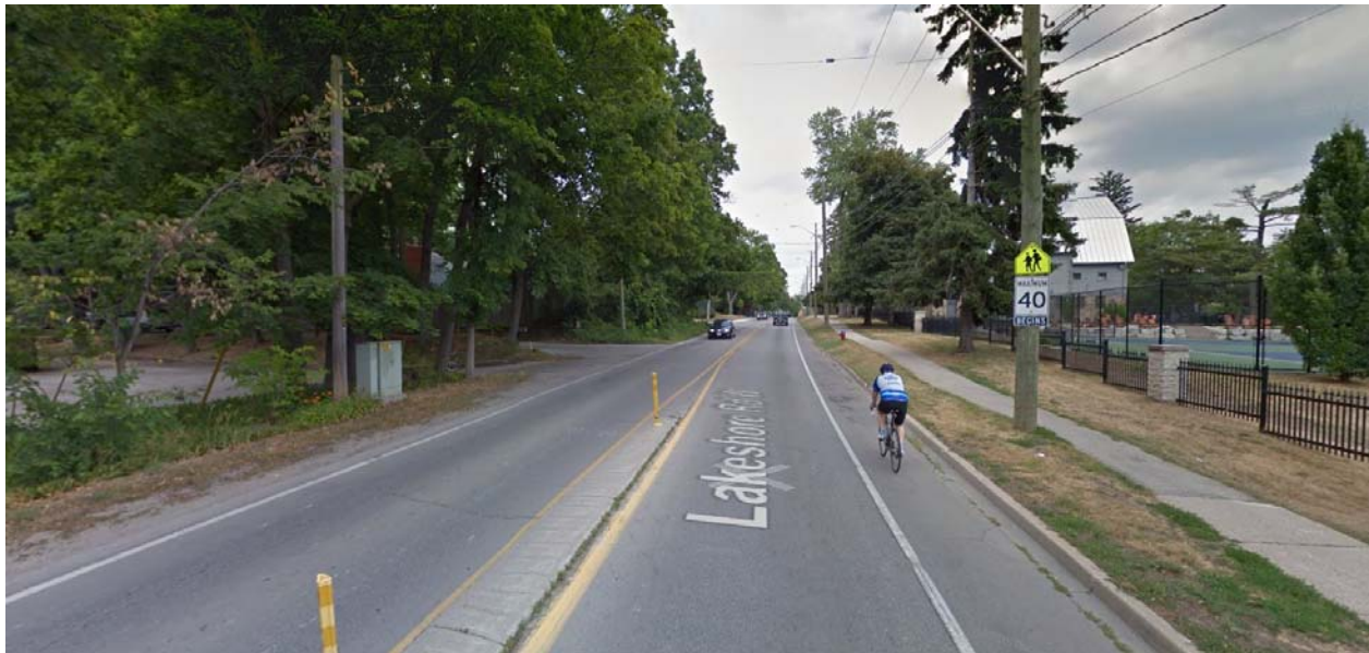
Figure 3.3. Undesignated Paved Shoulder Acting as a Cycle Lane
