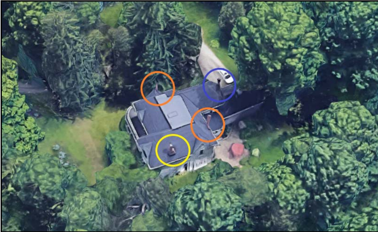
The yellow circle indicates a chimney in its known original location; the orange circles indicate chimneys likely moved after the 1905 fire and when the roof was enlarged; the blue chimney is likely in its historical location. Source: Google, edited
