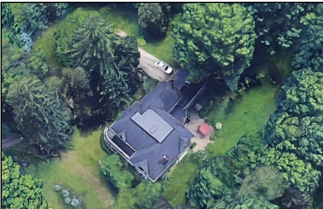
Google aerial showing the massing of the house, with the truncated hip roof on the main portion (the “L” on the west elevation is a peaked hip roof) and the further garage extension on the west/south elevation. Source: Google
