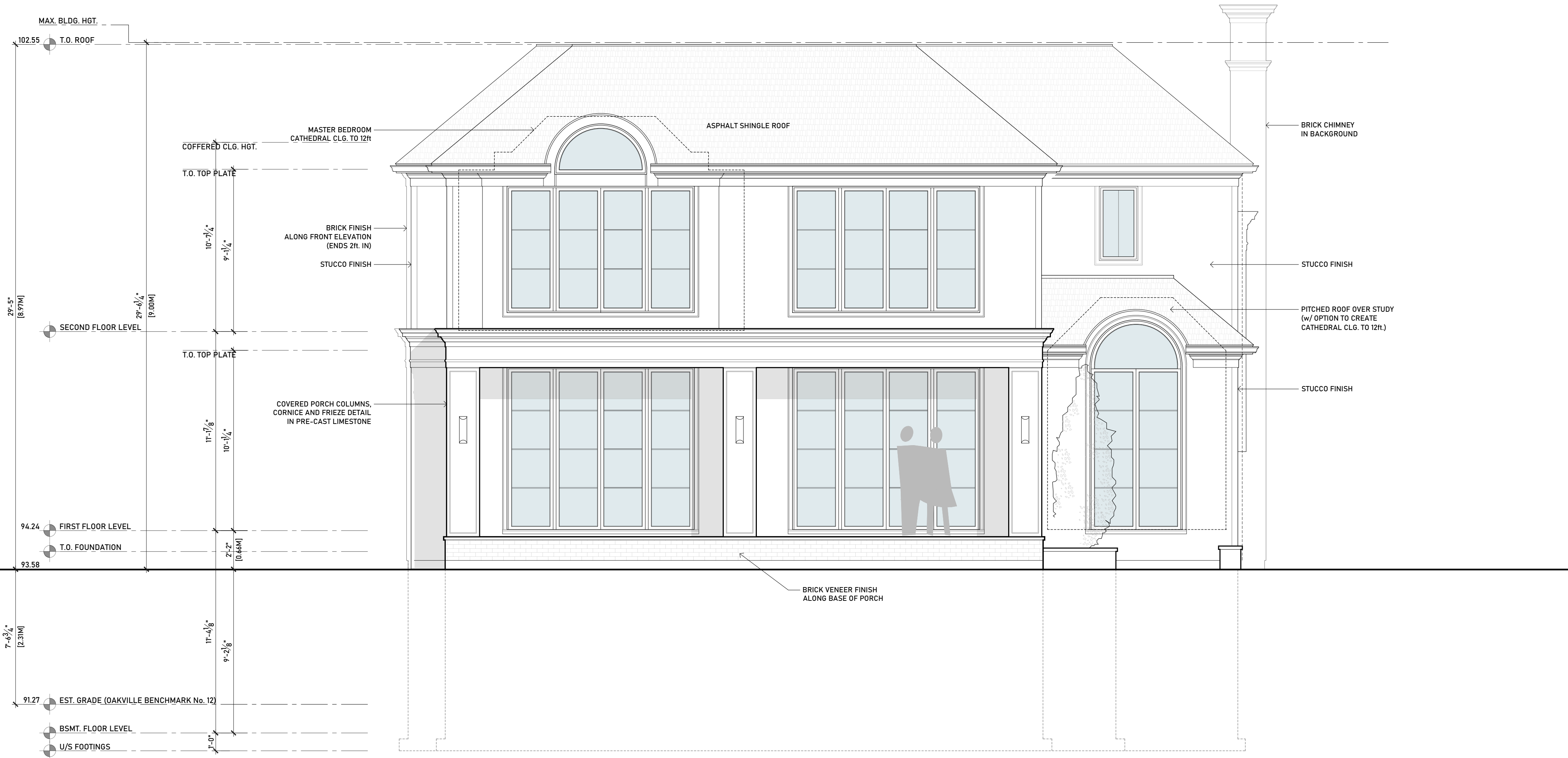
1 REAR (SOUTH) ELEVATION SCALE: 1/4" = 1'-0"
