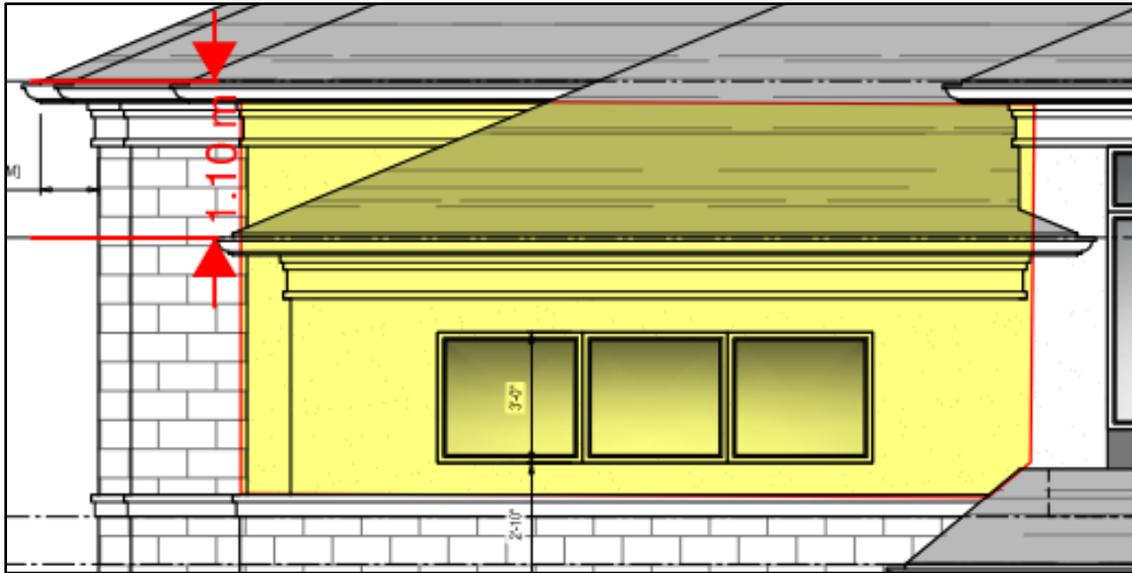
Figure 11: 2<sup>nd</sup> Storey rear roofline revision (2<sup>nd</sup> Submission)
