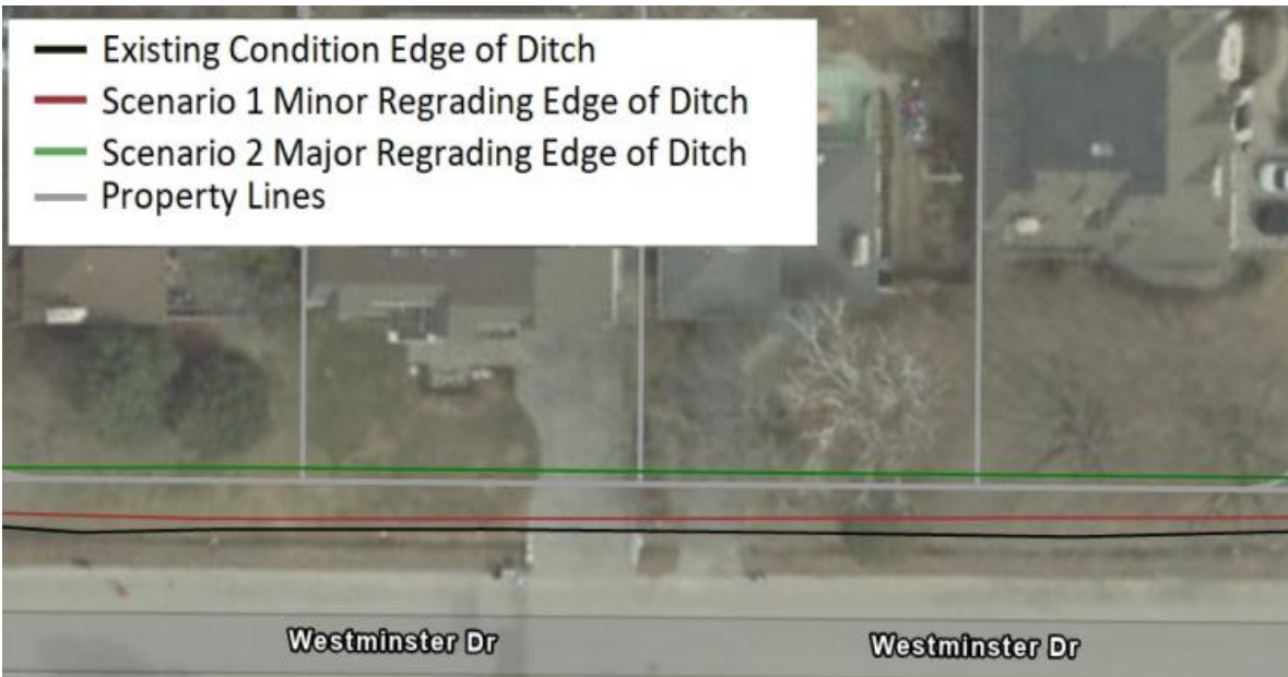
Exhibit C-5 –aerial view of extent of ditch limits for existing conditions, Scenario 1 and Scenario 2
