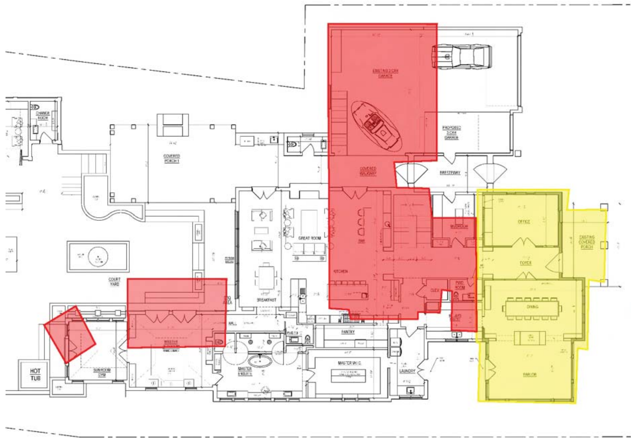
Figure 14: Portion to be retained over detail of the proposed floor plan. Yellow to be retained. Red to be removed (approximate)
