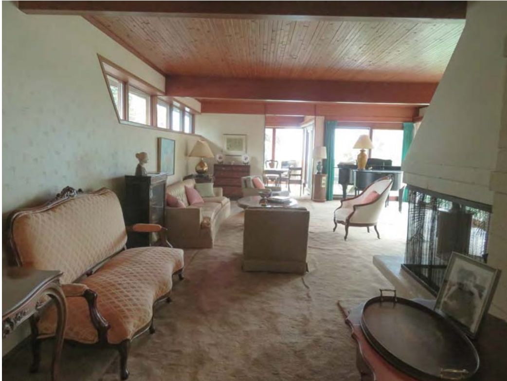
LIVING ROOM – EXPOSED MASONRY WALLS – EXPOSED WOOD BEAMS AND WOOD CEILINGS – WALL TO WALL CARPET – ARCHITECTURAL FIREPLACE – PLYWOOD & GYPROCK PARTITION WALLS
