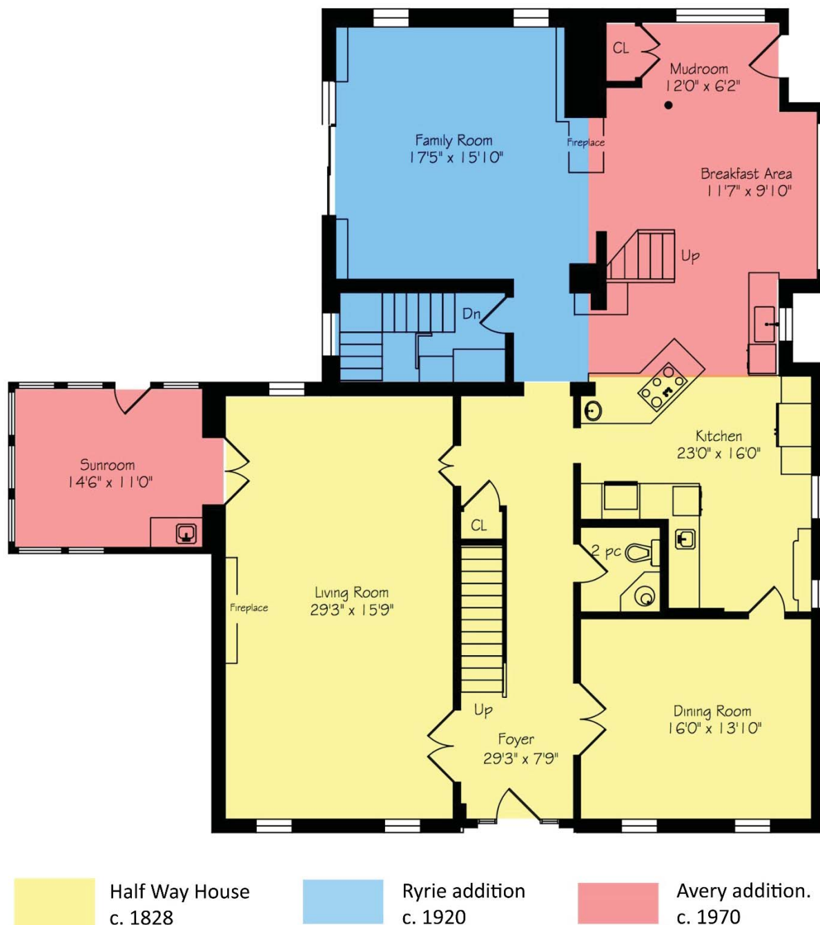
Figure 52: Ground Floor Plan showing original house and later additions Credit: Client-provided floor plan with SBA annotation
