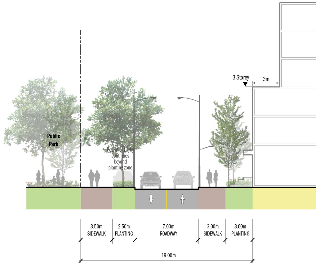
Figure 33. Potential Street Section for Private Street
