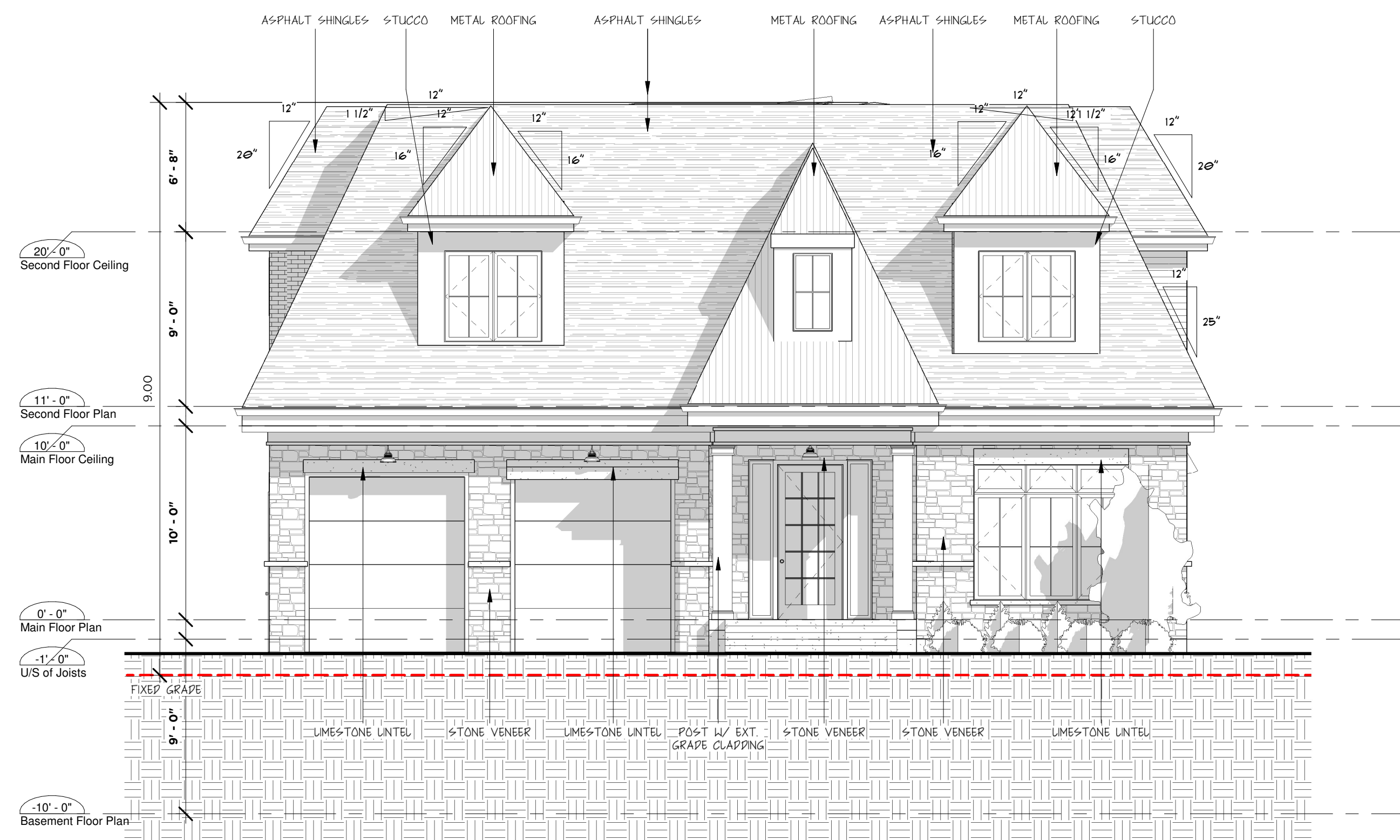
1 Proposed South Elevation 3/16" = 1'-0"
