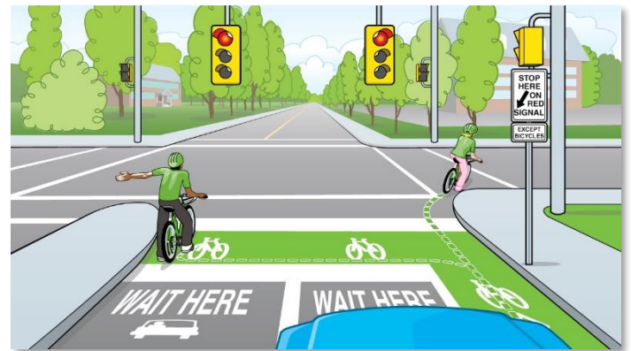
Figure 5-3: Bike-Box Cycling Configuration at Intersections
