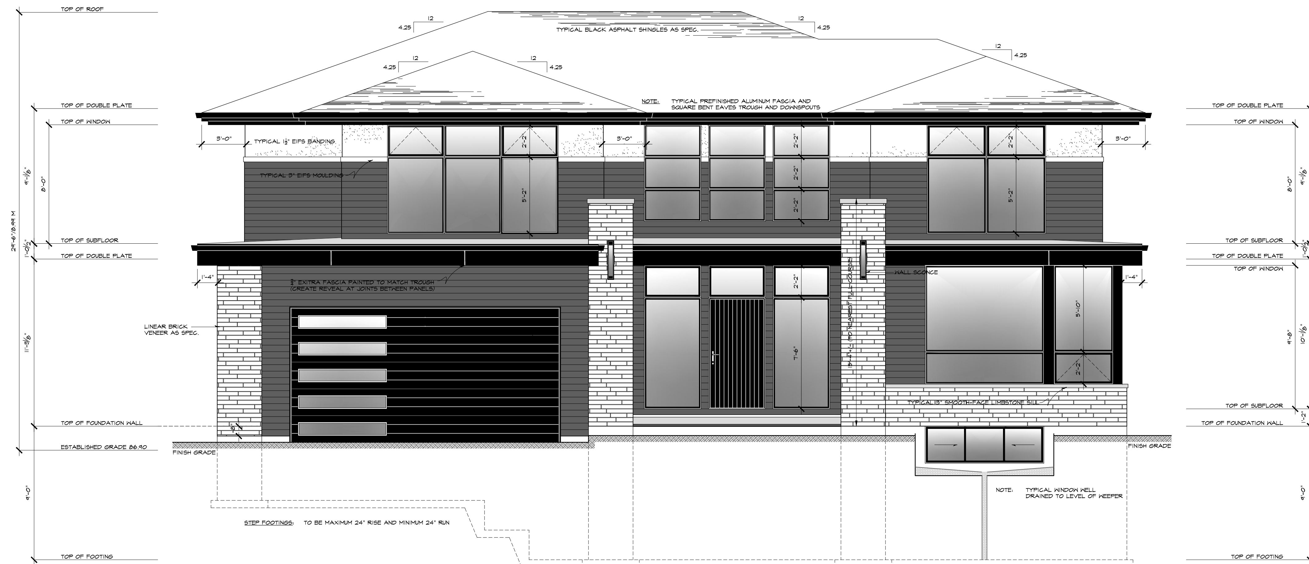
1 A07 NORTHEAST ELEVATION SCALE: AS NOTED
