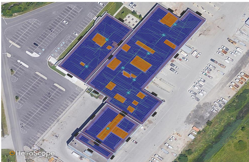
Figure 9: Conceptual roof PV array at 594 \text{ kW}_{AC} ( 718 \text{ kW}_{DC} )
